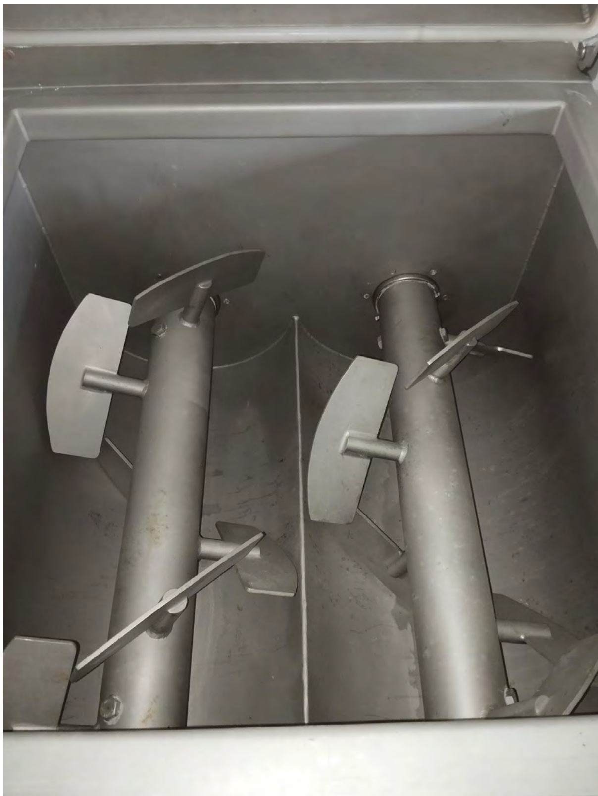
Mixer from inside - for mixing Meat and other ingredients
