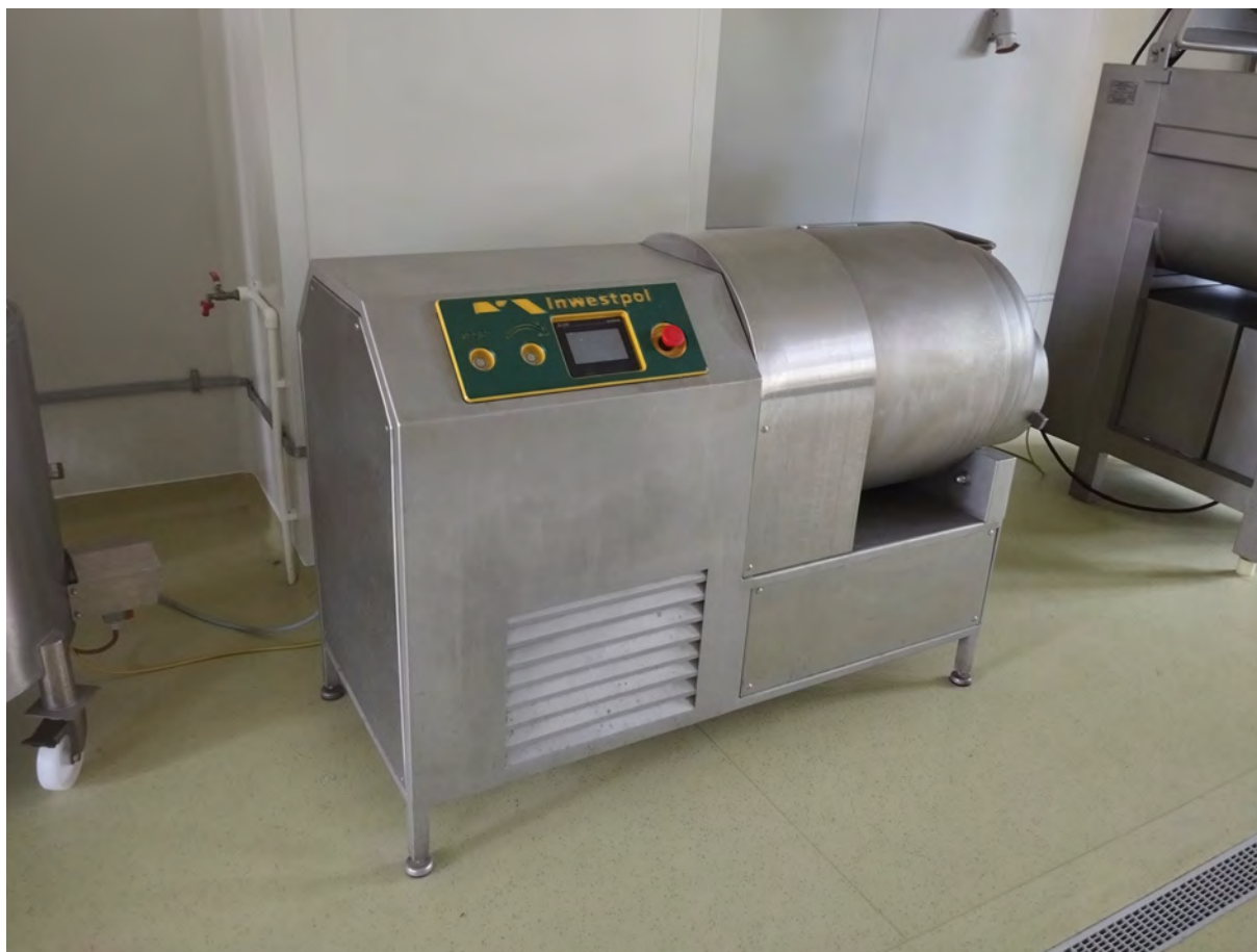
Tumbler for Protein activation after brine injection in Meat pieces for cooked ham
