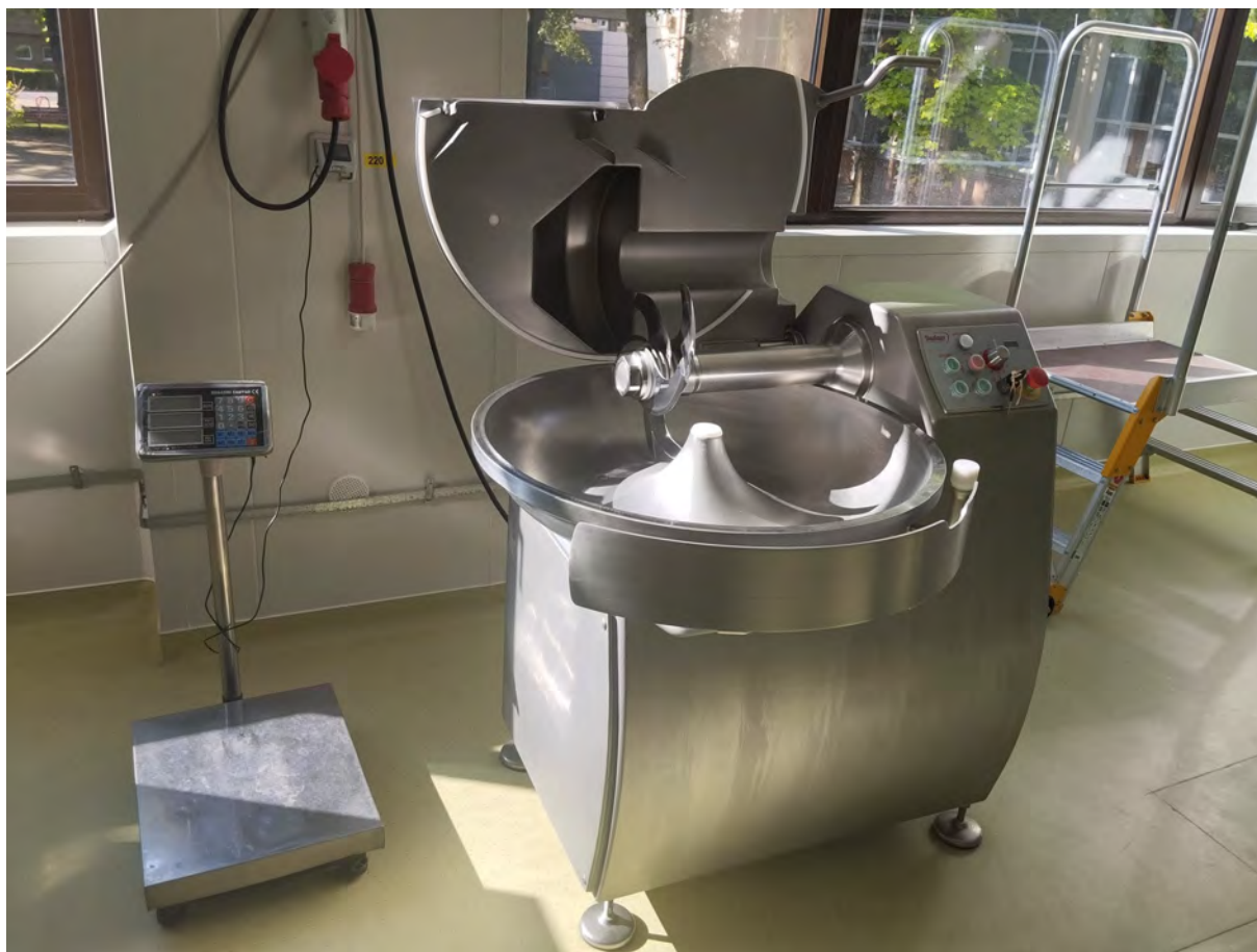
Cutter for Meat – to prepare Emulsion for Boild Sausage
